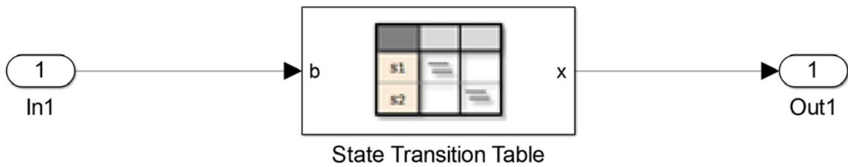
Fig 3. Layout of Simulink – state flow model (i.e., “In1” represents “b” and “Out1” represents “x”)
