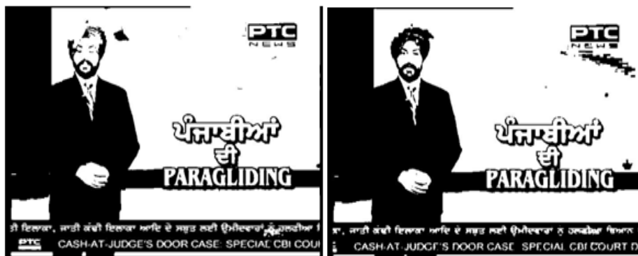
Fig. 3. Binarization using Otsu method in DotNet (left) and MATLAB (right)
