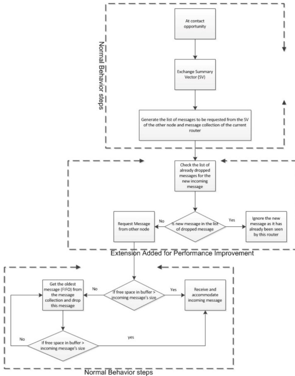
Figure 2: Extended behavior of router with Epidemic Routing protocol in DTN.
