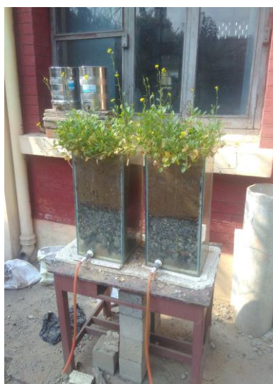
FIGURE 1. VERTICAL SUB-SURFACE FLOW CW MODEL
