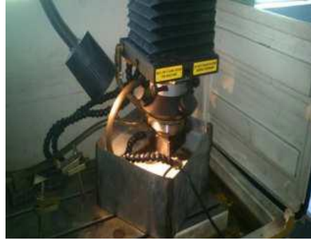
Fig. 3 Small working tank and jet flushing system used in the EDM process
