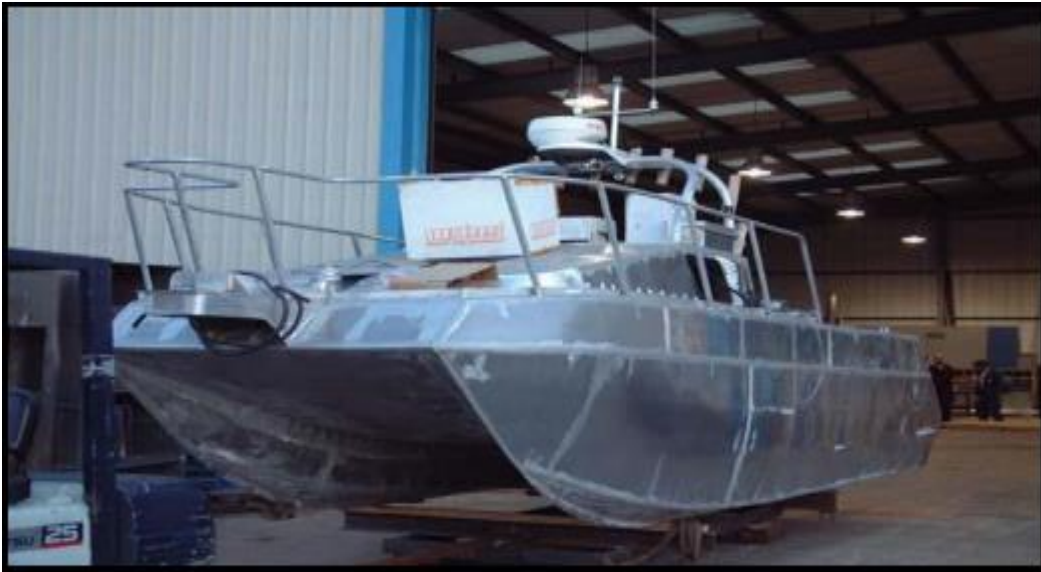
Fig. 4 FSW used in Ship building
