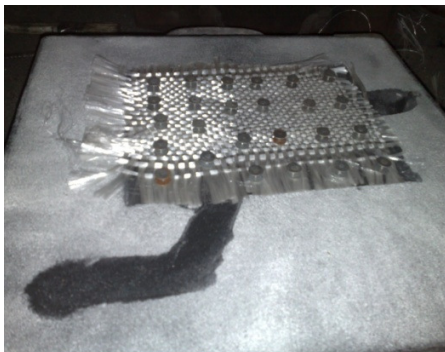
Fig 3.1(c): Placing of fibre
