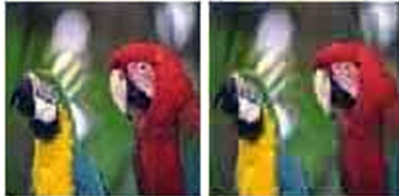
Figure 4.2: Original image 'Parrots.jpg' with 8806 colors on left and Quantized image 'Parrots.jpg' with 5503 colors on right.
