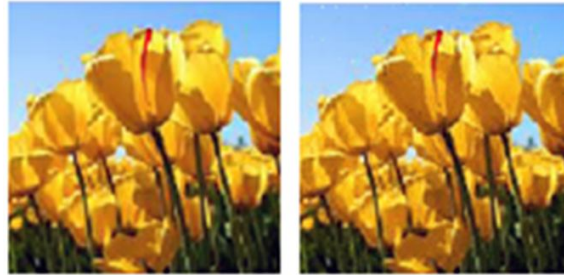
Figure 4.6: Original image ‘Image2.png’ with 8824 colors on left side and Quantized image ‘Image2.png’ with 5740 colors right side.
